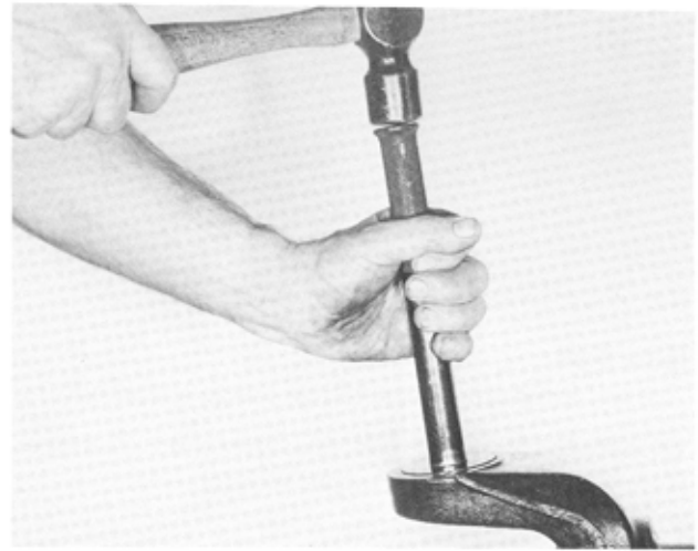
Figure 3-31 Assemble new grease retainer and king pin bearing cup.
