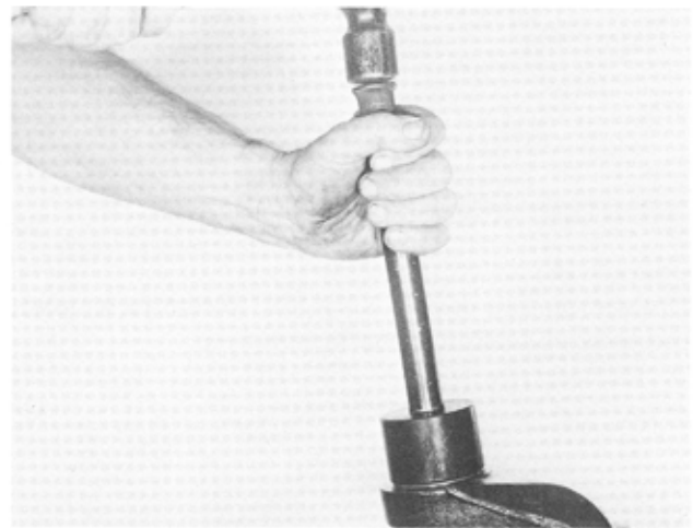
Figure 3-32 Fill the area in grease retainer with specified grease, grease bearing cone and install. Install new king pin bearing oil seal.
