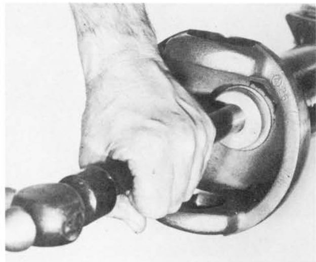
Figure 3-12 Assemble new bronze bushing into ball yoke. TOOLS: D-161 Installer C-4171 Handle
