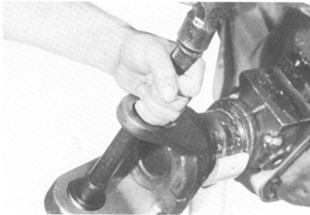
Figure 3-30 Remove king pin bearing cup, cone, grease retainer, and seal all at the same time. Assemble and use tools exactly as shown. Discard seal and replace with new one at time of assembly. If grease retainer is damaged, replace with new one at time of assembly.
