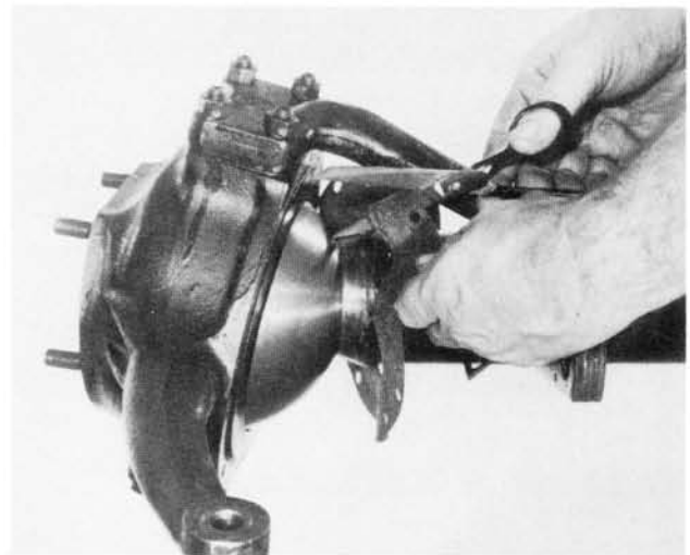
Figure 3-4 Cut felt in half to disassemble. Discard felt seal.
